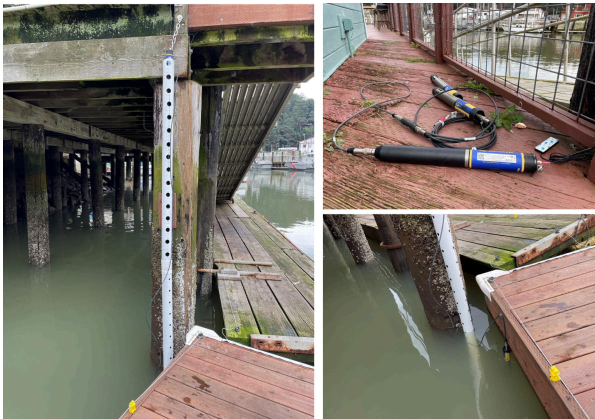
Figure 4: Set-up of water quality instrumentation at the Noyo Center Marine Field Station. Left: Perforated PVC pipe containing battery for telemetry system at the top and bottom sensor fixed two feet from the seafloor. Top Right: AquaTroll 500 Multiparameter Sondes with battery, manufactured by In-Situ. Bottom Right: Surface sensor hanging from floating dock.
