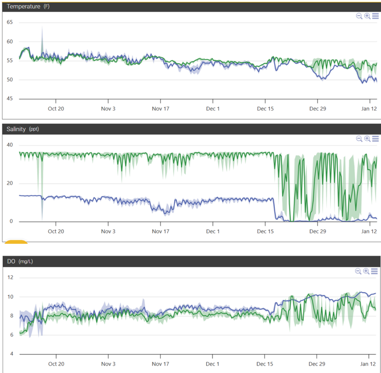
Figure 39: Temperature, salinity, and dissolved oxygen from October 11, 2025 to January 12, 2026. The green line is the bottom sensor and the blue line is the surface sensor.
